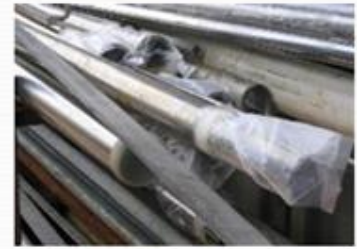
•End seal for pipelines not in use
