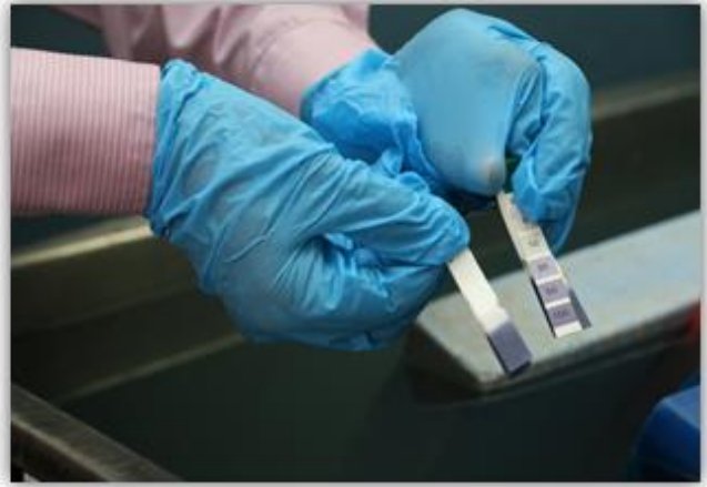
Checking strength of chlorine (100-200 ppm) water using chlorine strips
