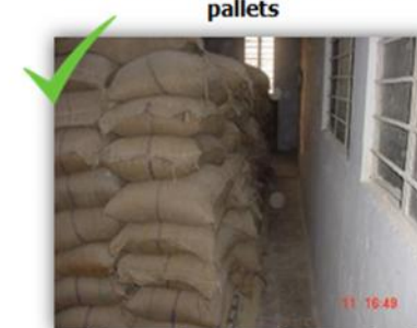
Proper stacking of raw material away from wall
